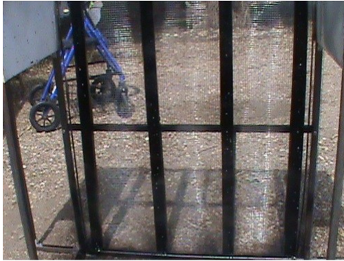
Added supports to basket bottom and treated with asphalt undercoating
