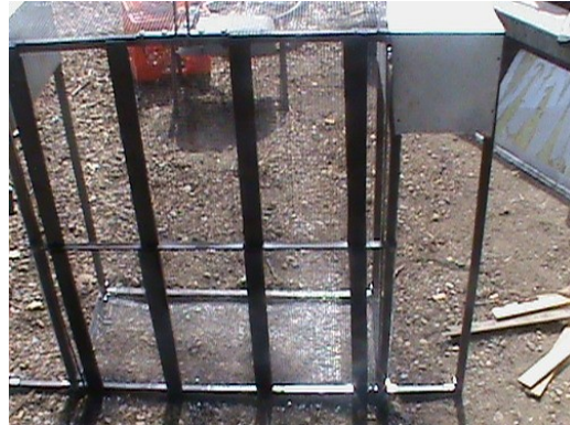
Added supports to basket bottom and treated with asphalt undercoating
