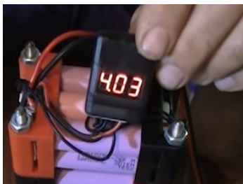
Cell loggers check voltages
