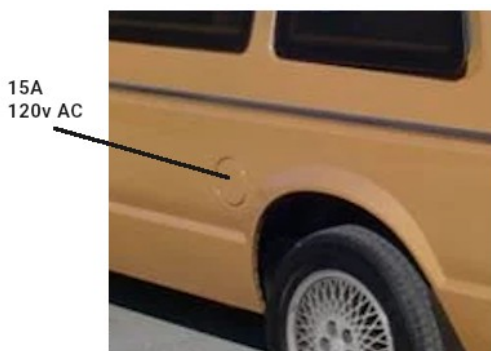
EV charge port behind old gas filler cap
